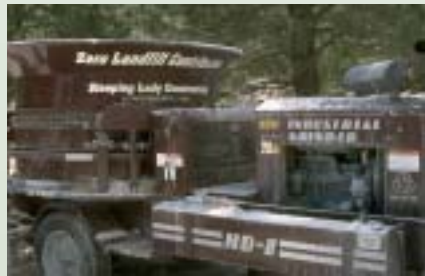
wood waste grinder
